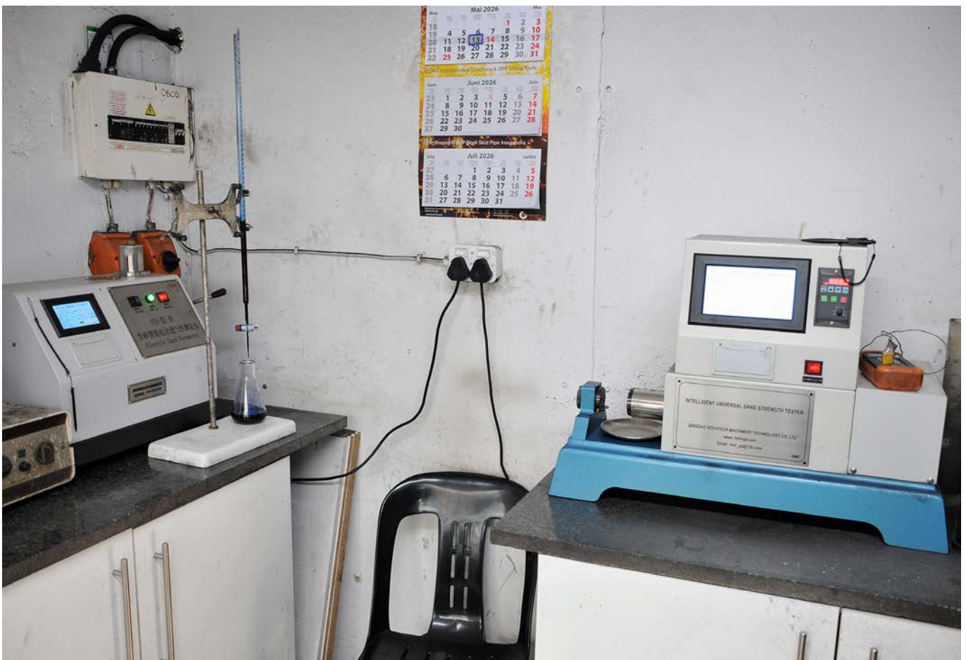
Recognising that green sand quality is fundamental to casting performance, Malleable Castings invested in upgraded laboratory testing equipment, including a green sand universal tester and a permeability tester
