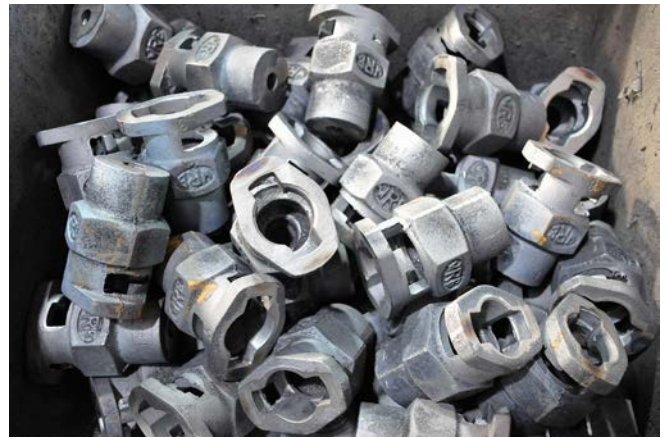
Currently Malleable Castings are processing 5 high-volume ductile iron components on the automated 5-axis fettling machine and a second machine is scheduled for installation in June 2026. One operator will run both machines and that includes loading and unloading
