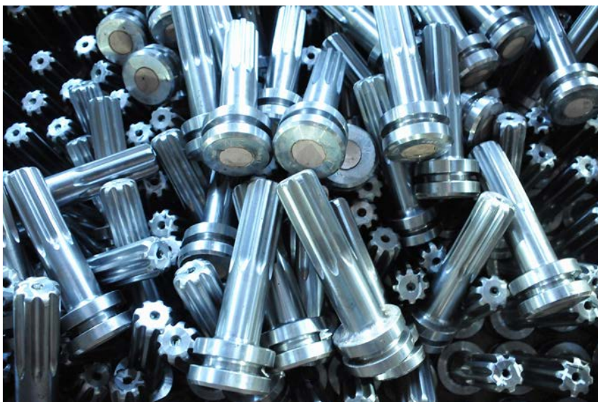
P.H. Heat Treatment offers stress relieving, annealing, normalising, hardening, tempering, blackening, carbon restoration, case hardening (carburising; carbonitriding; lamda processes) and gas nitriding
