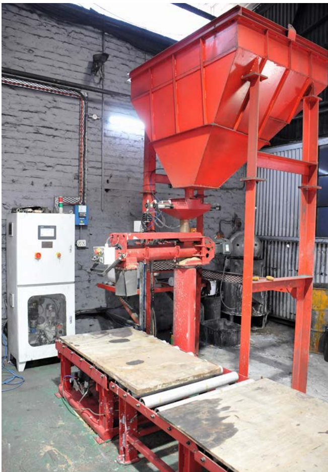
Malleable Castings has also invested in a 2-ton an hour continuous mixer for alkaline phenolic no-bake moulding, enabling the foundry to manufacture larger castings beyond the dimensional limits of its green sand operation
