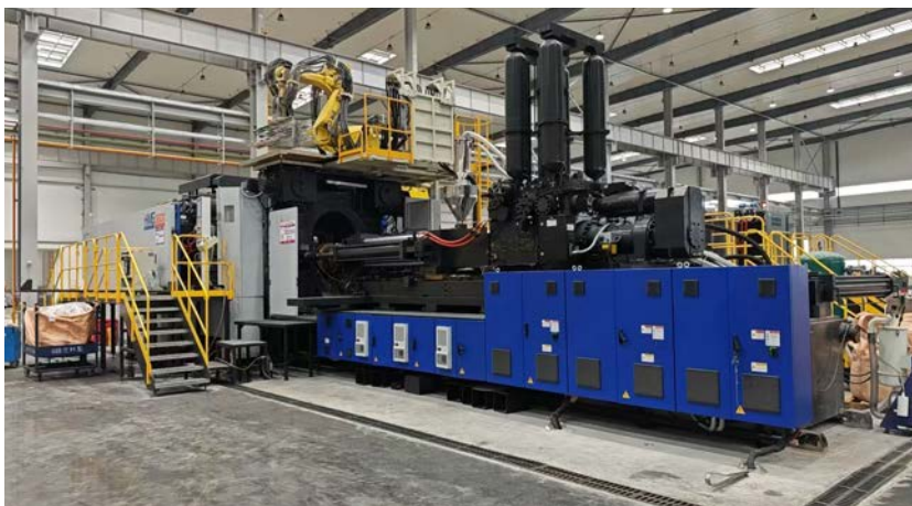
The world's first mass-produced semi-solid process magnesium alloy body component was produced on the HMG3600 large-scale magnesium alloy injection moulding machine
