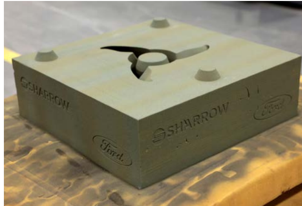
Ford and Sharrow have worked to adapt Sharrow's propeller designs to a 3D printed sand-casting process, refining and validating the approach for high-volume output
